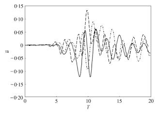
Figure 8. Time history of the displacement at  $(z = 10.0, \theta = 0)$  on the outer surface of Type 1 shell  $(R_1 = H)$  excited by an incident wave at  $(z = 0.0, \theta = 0)$ . (n = 1.0; (-1.1), (n = 2.0; -..., n = 4.0).
