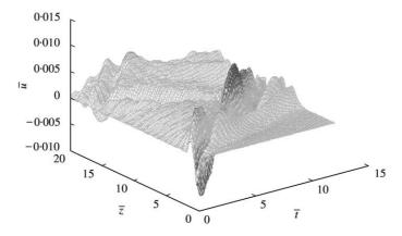
Figure 11. Displacement u on the outer surface in the z-t plane of Type 2 cylindrical shell  $(R_1/H = 20)$ .
