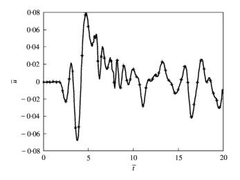
Figure 3. The time history of the displacement at z = 5H on the upper surface on the SiC-C FGM plate excited by an incident wave of one cycle of sine functions at z = 0: —, present method; \_\_\_\_, Liu *et al.* (1999).
