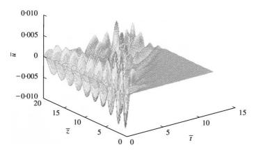
Figure 9. Displacement u on the outer surface in the z-t plane of Type 1 cylindrical shell  $(R_1/H = 20)$ .
