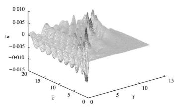
Figure 12. Displacement u on the outer surface in the z-t plane of Type 3 cylindrical shell ( $R_1/H = 20$ ).
