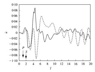
Figure 14. Comparison of time history of displacement u on the outer surface at z = 2H subjected to a vertical line load with a time history of one cycle of sine function at x = 0 (-----, stainless steel shell; - - -, Type 1 shell (n = 1)).
