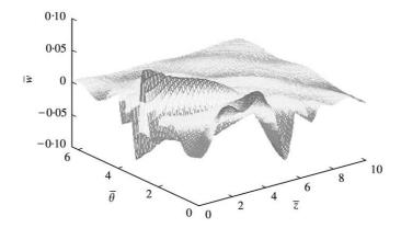
Figure 4. The response distribution of the radial displacement w on the outer surface of Type 1 shell  $(R_1 = H)$  subjected to a radial point load at  $(z = 0, \theta = 0)$  with a time history of one-cycle sine function.
