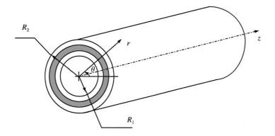
Figure 1. Configuration of an FGM shell.
