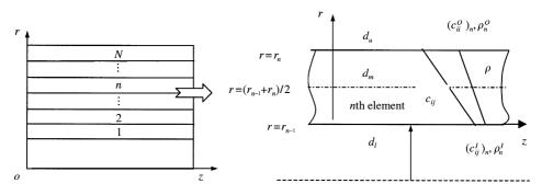
Figure 2. Annular element subdivision and the *n*th isolated annular element.
